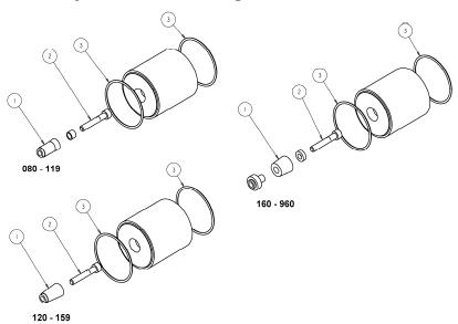
Figure 49 PR70 Nylon and UHMWPE Piston Replacement Kits
